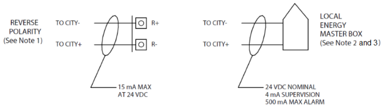
Figure 28: City card wiring
